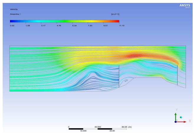
The usual design of wind protection systems is based on fix structures for net installation that has to reduce the wind velocity and eliminate wind turbolences in the curve of jumping. Structures are assembled before the start of tournament and disassembled after ski jumping is finished.
